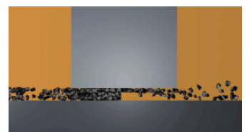
CONTAMINATION IN PRESENCE OF NARROW TOLERANCES
